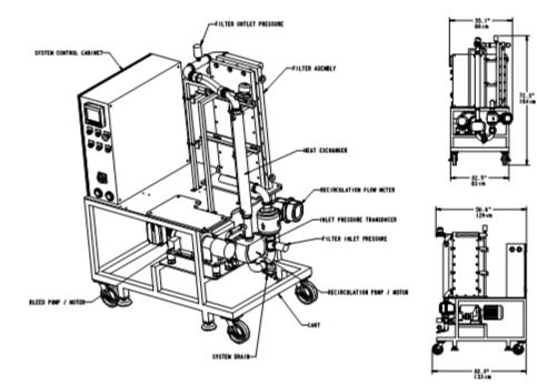
The Infinity on this page includes the OPTISEP 11000 in a feed and bleed configuration for process development and low volume production with volumes from 15 to 500 Liters.
